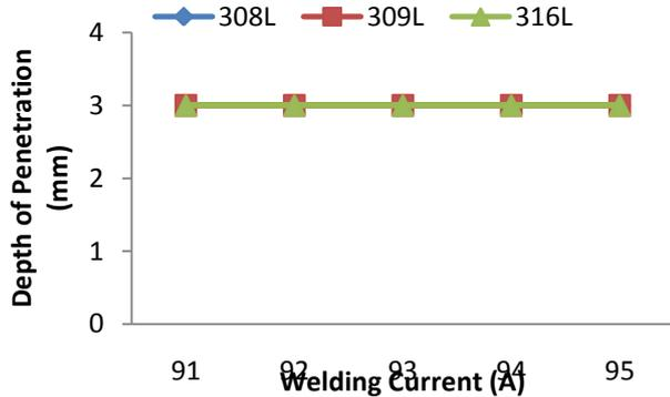
Fig.1. Effect of welding current and filler metal type on weld penetration
