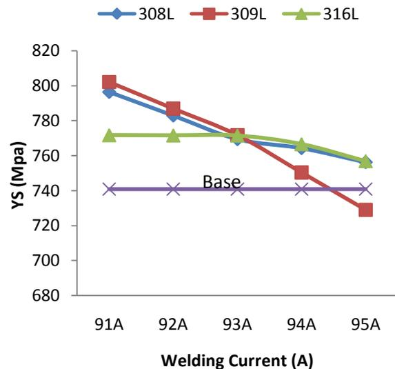
Fig.5. Effect of Welding Current on Ultimate Tensile-Strength of Welded Joint
