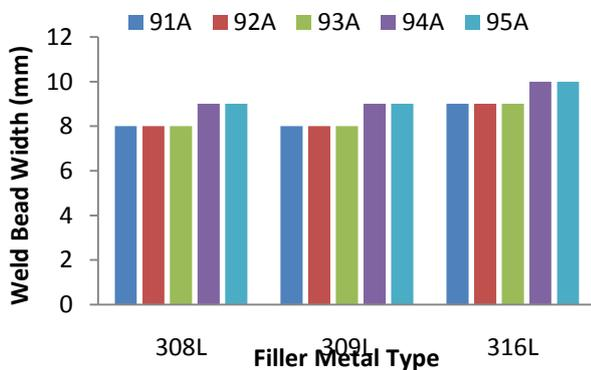
Fig.3. Effect of Filler Metal Type on Weld Bead Width
