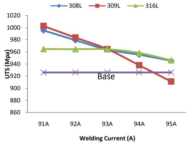
Fig.4. Effect of Welding Current on Yield Strength of Welded Joint
