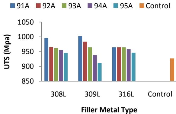
Fig.6. Effect of Filler Metal Type on Ultimate Tensile Strength of Welded Joint
