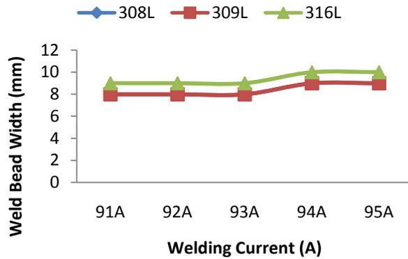
Fig.2. Effect of Welding Current on Weld Bead Width
