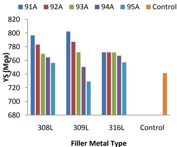
Fig.7. Effect of Filler Metal Type on Yield Strength of Welded Joint
