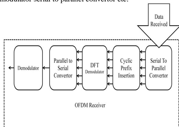
Fig.2. Receiver of OFDM
