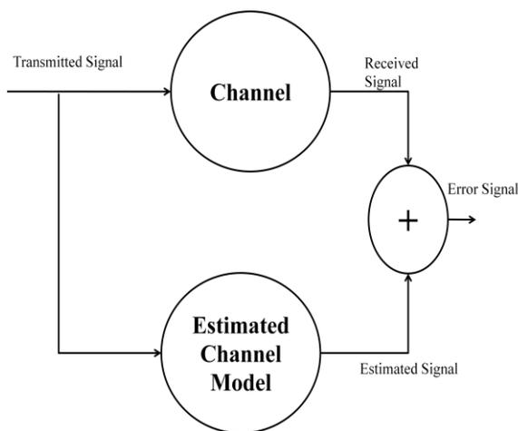
Fig.3. Channel Estimation Sequence
