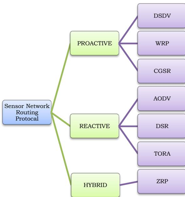
Fig.2. Hierarchy of Routing Protocol
