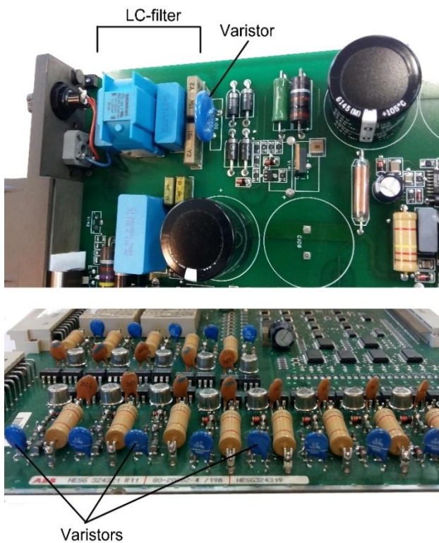
Fig.10. Usage varistors in power supply (up) and logic inputs (down) of relay protection
