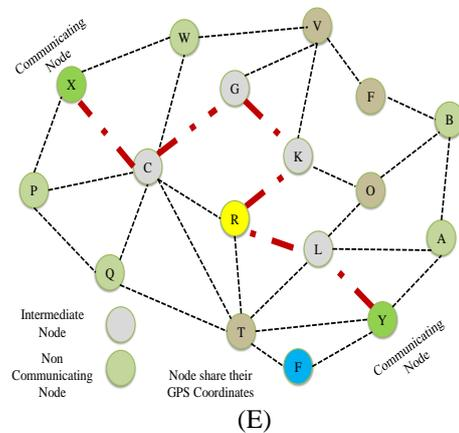
The RERR message provides information about the link failure and the alternative route between the node that generated the route error packet and the receiving node. Same process is repeated for node F and O. Finally node F is selected for supplement support after applying ARAODV.
