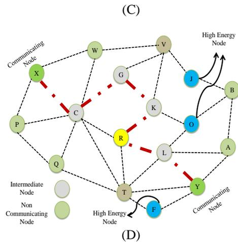
Whereas node P broadcast node supplement request packet over the network and node F, O and J reply for that. Node J checks its routing table to find the alternative path from node J to sink node and select the best route between the paths to sink node. Then node J generates and sends the RERR message to the source node.
