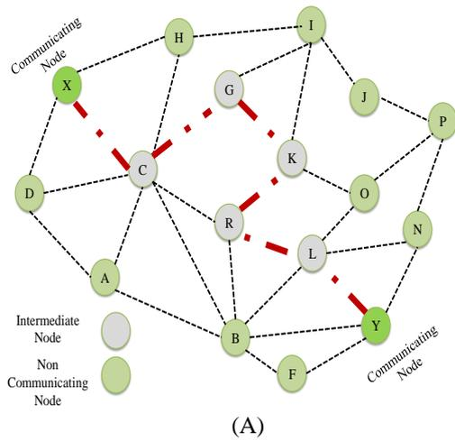
When node R drop their energy level below threshold then it broadcast responsibility overtake packet to their radio node and perform voting for responsibility overtake as show in figure.1(b) and chose on the basis of node having enough energy to transmit the packet and having lower load currently as case B. And simultaneously node before R node ie Node K transmits that packet from alternate Route as shown in figure 1(C) as case C.
