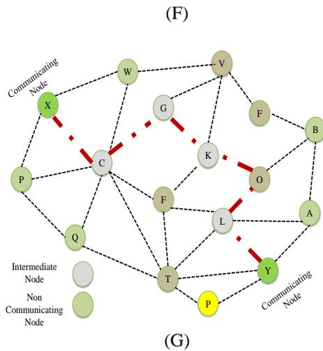
Fig.1. Route Construction Phase in ESAODV
